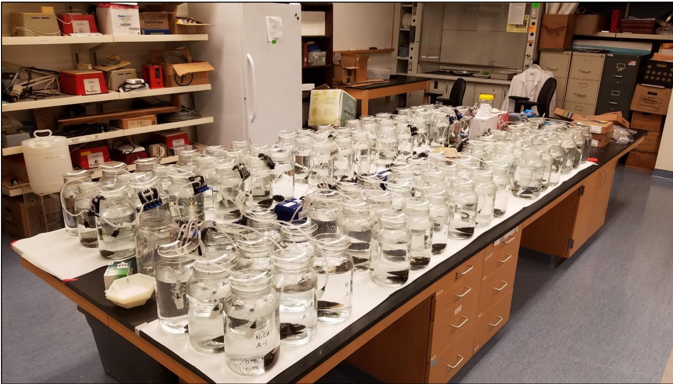
Figure 1. Photograph of experimental set up and aerated static-renewal design, with nine replicate aquaria in each of five metal treatments, and one mussel per aquarium (two experiments shown, one on either side of the lab bench).
