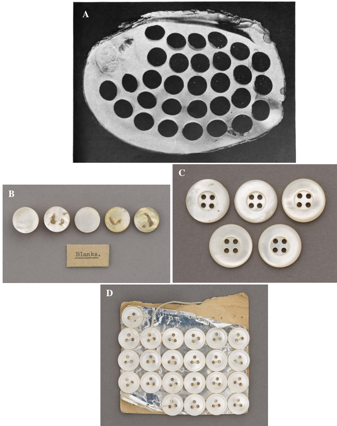
Figure 3. (A) A drilled Washboard ( Megalonaias nervosa ) mussel shell drilled for button blanks, (B) button blanks, (C) finished buttons, and (D) carded buttons ready for market. [(A) From RE Coker. 1919. Fresh-water mussels and mussel industries of the United States. Bulletin of Fisheries, Volume 36. (B-D) from the courtesy of the Birmingham Museum and Art Gallery via Flickr Creative Commons.]
